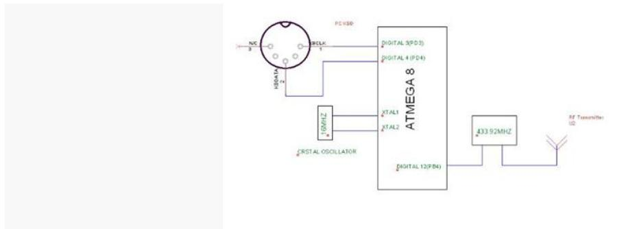
Schematic of the Transmitter
