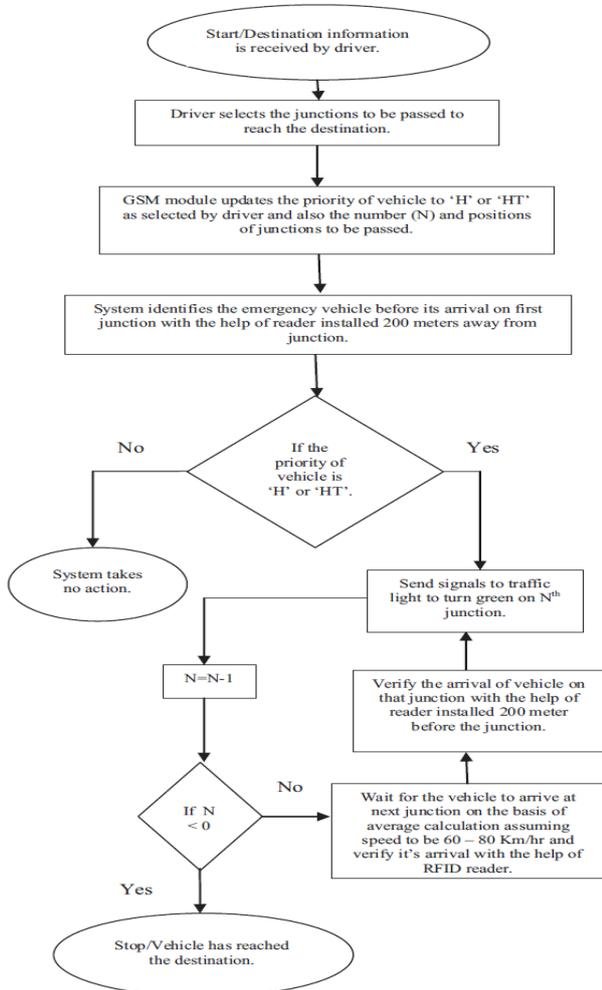
**Fig 3 Flow of Software for Green wave**
