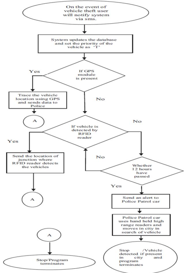
**Fig 4 Flow of Software for Detection of Stolen vehicles**
