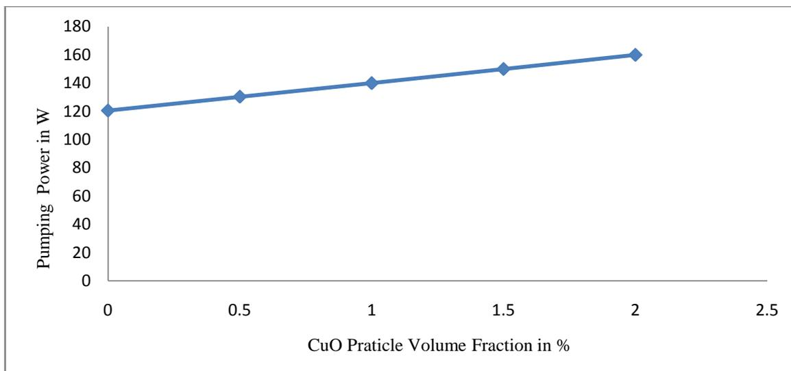
**Fig No 6** Variations of Pumping Power for nanofluid at different volume fractions
