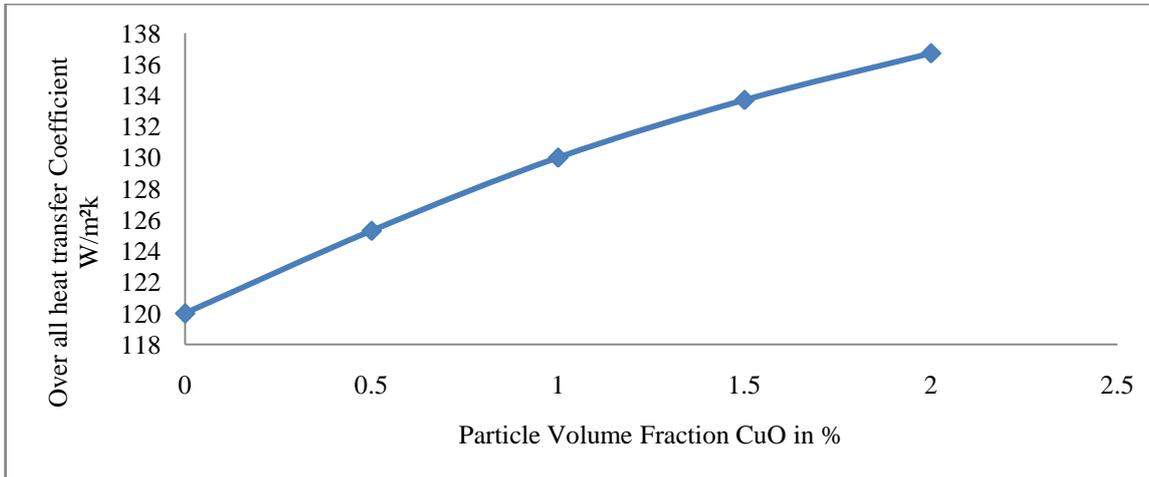
**Fig No 3** Variations of Overall heat transfer coefficient for nanofluid at different volume fractions.
