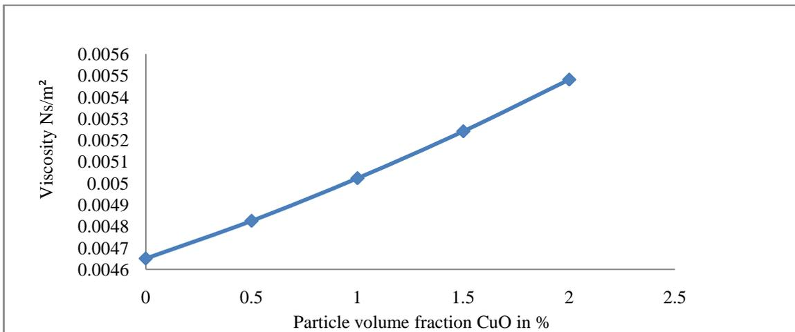
**Fig No 2** Variations of Viscosity for Nanofluid at different Particle fraction
