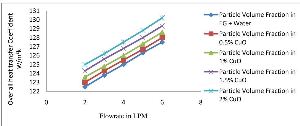
**Fig No 4** Variation of Overall heat transfer coefficient for nanofluid at different flowrate in (LPM).
