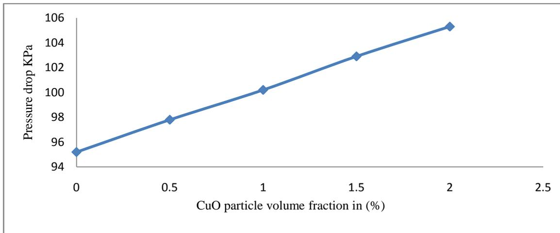
**Fig No 5** Variations of Pressure drop for nanofluid at different volume fractions
