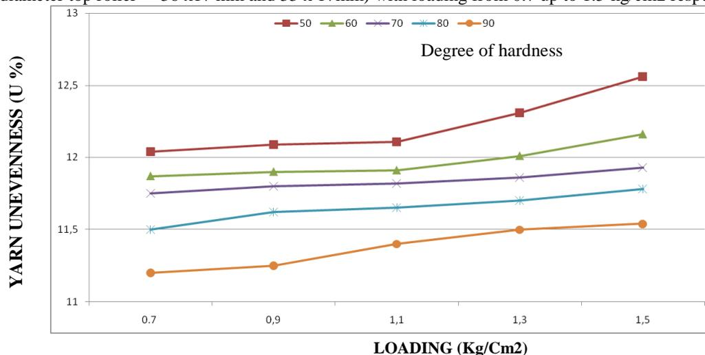
Figure 6. The relationship between degree of hardness, loading and the result of yarn unevenness (U %) (Diameter : 36x17 , 29.55Tex)
