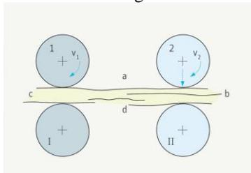
Figure 1. The floating fibers (d), Guided fibers (a,b and c)
