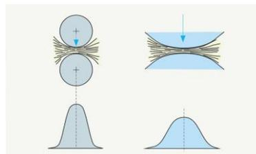
Figure 5. Effect of diameter rubber rollers
