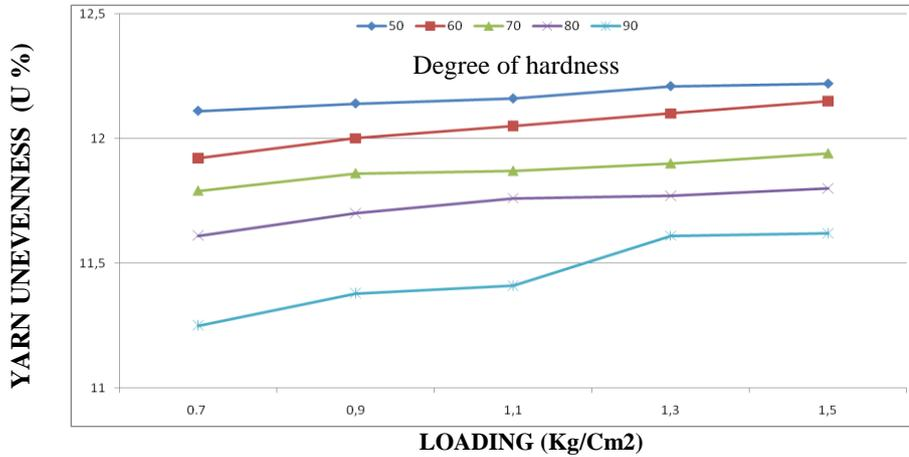
Figure 9. The relationship between degree of hardness, loading and the result of yarn unevenness (U %) (Diameter : 33x17 , 29.55Tex)
