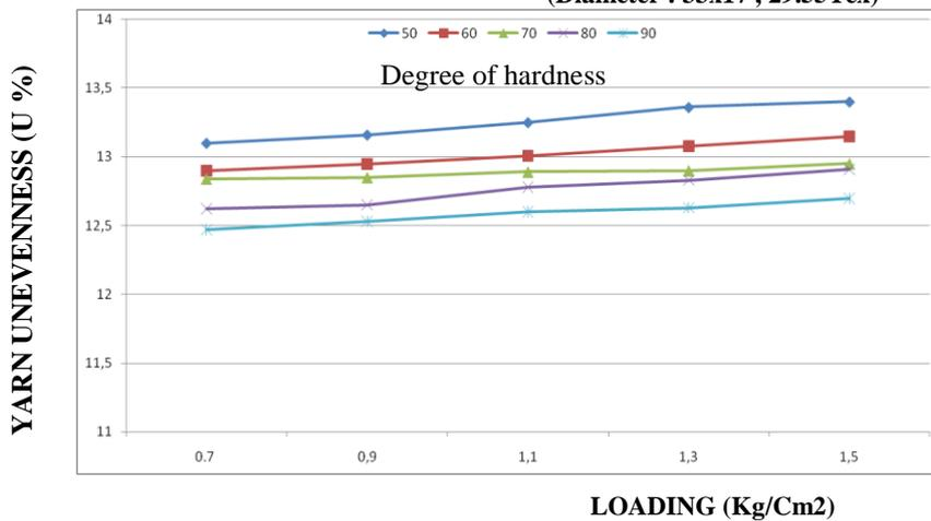
Figure 10. The relationship between degree of hardness, loading and the result of yarn unevenness (U %) (Diameter : 33x17 , 13.13Tex)
