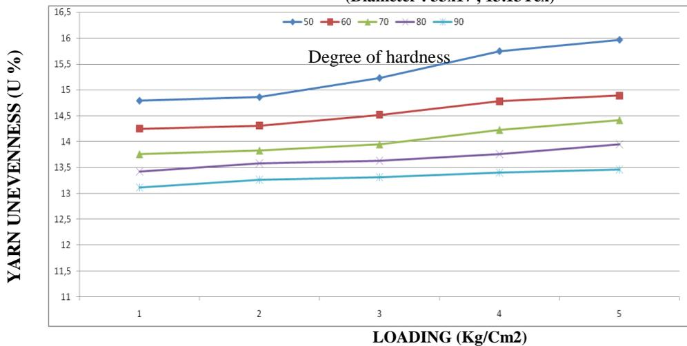
Figure 11. The relationship between degree of hardness, loading and the result of yarn unevenness (U %) (Diameter : 33x17, 9.8Tex)
