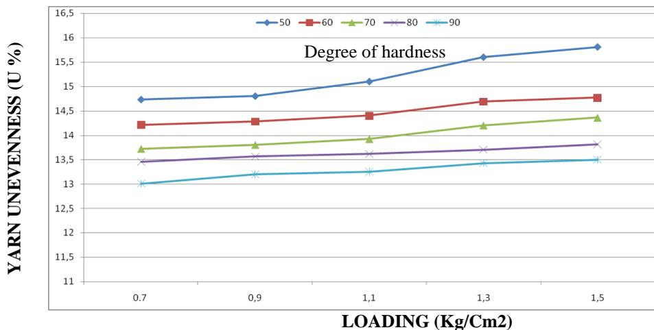
**Figure 8. The relationship between degree of hardness, loading and the result of yarn unevenness(U %) (Diameter : 36x17 , 9.8Tex)**
