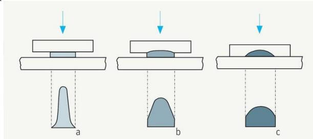
Figure 4. High roller pressure causes strong compression
