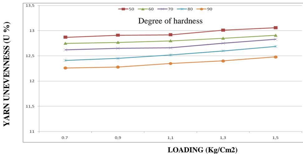
**Figure 7. The relationship between degree of hardness, loading and the result of yarn unevenness (U %) (Diameter : 36x17 , 13.13Tex)**
