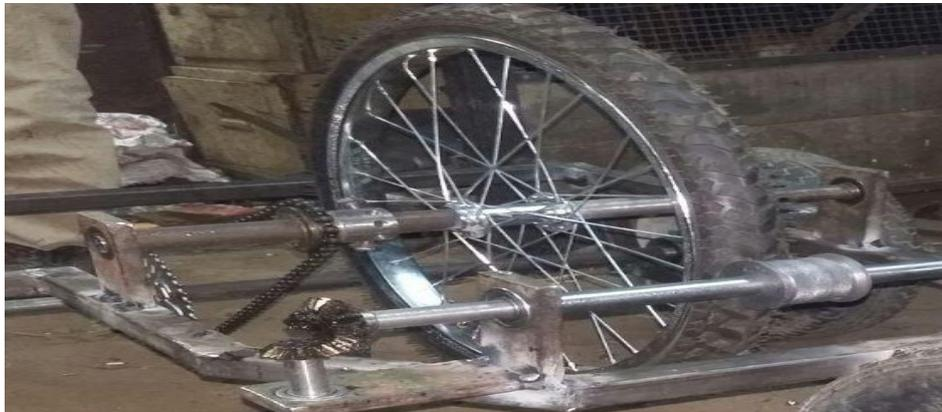
Fig 3: Power transmission system
