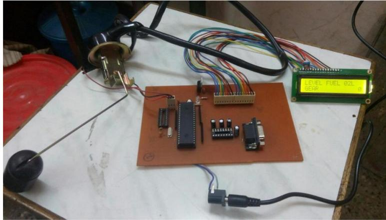
**Figure 4: digital fuel meter kit**
