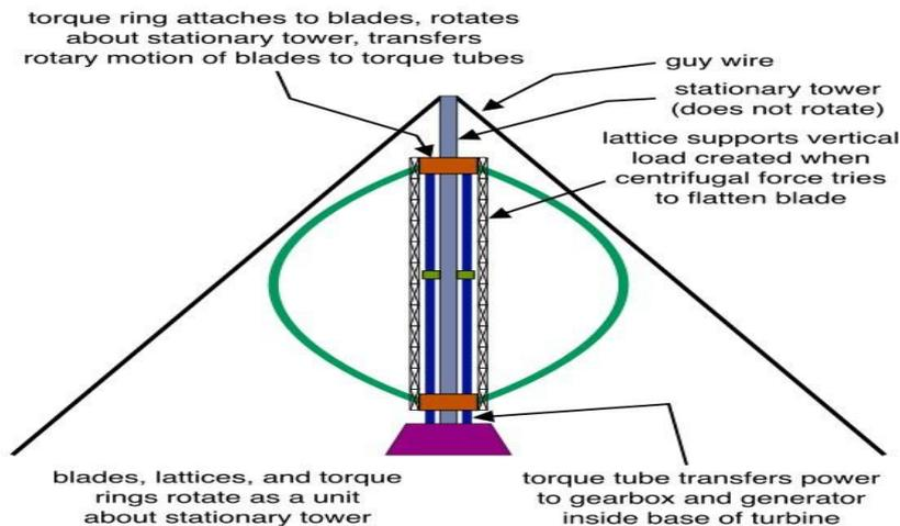
**Figure 3: High Mechanical Efficiency Centrifugally Stable Darrieus Turbine**
