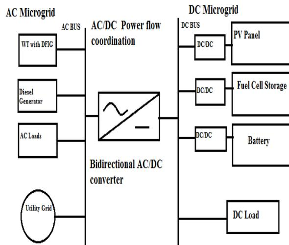
FIG3: Schematic diagram of hybrid AC/DC micro-grid.
