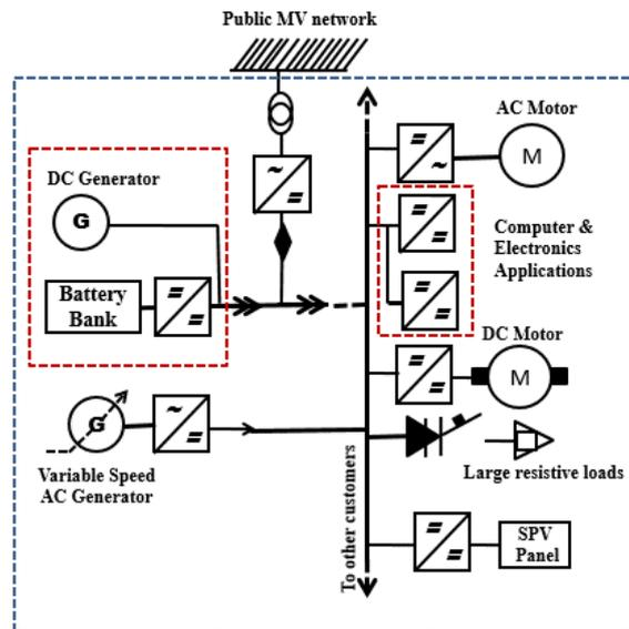
FIG 2: Schematic diagram of DC Micro-Grid.
