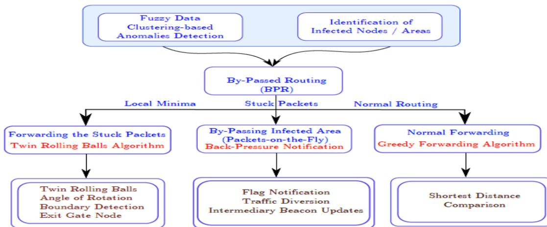
Fig 4 The proposed architecture view[BPR technique]
