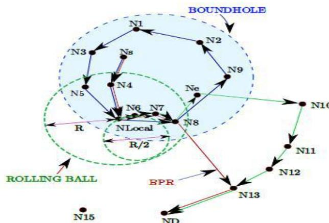
**Fig 6 Example of constructing path using Rolling ball technique**
