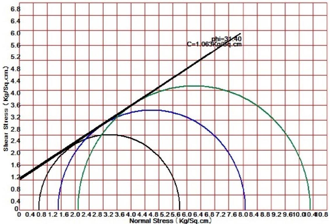
**Figure 7 Mohr's Circle For Triaxial Test (Soil=100%,FC=0.3%,FL=12mm)**
