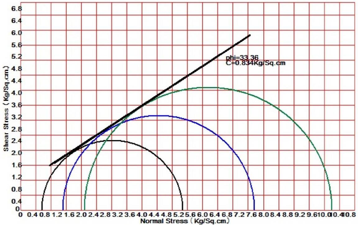
Figure 5 Mohr's Circle For Triaxial Test (Soil=100%,FC=0.1%,FL=12mm)
