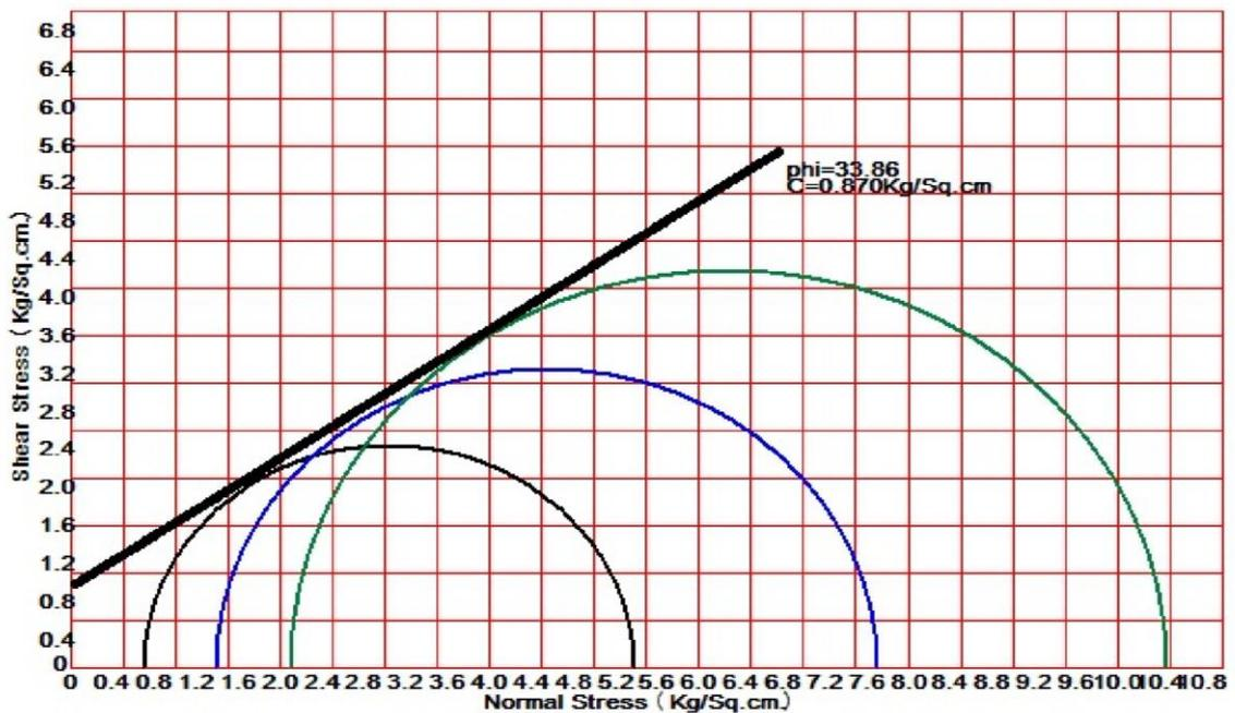
Figure 6 Mohr's Circle For Triaxial Test (Soil=100%,FC=0.2%,FL=12mm)
