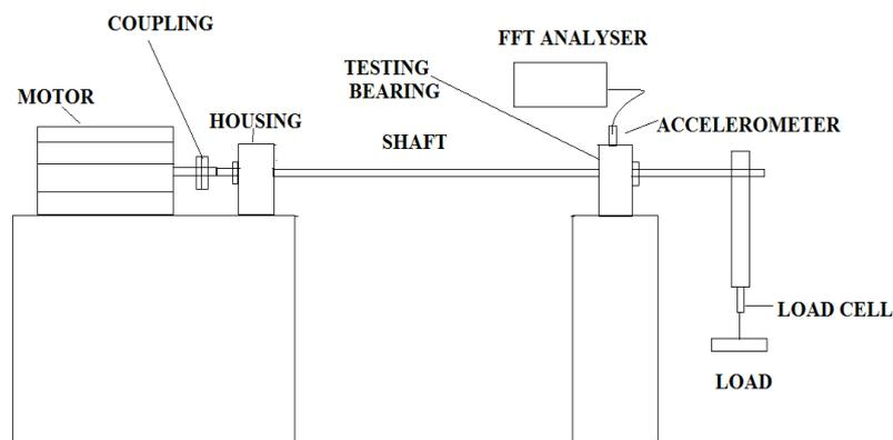
FIG . 01- EXPERIMENTAL SETUP FOR PROPOSED WORK
