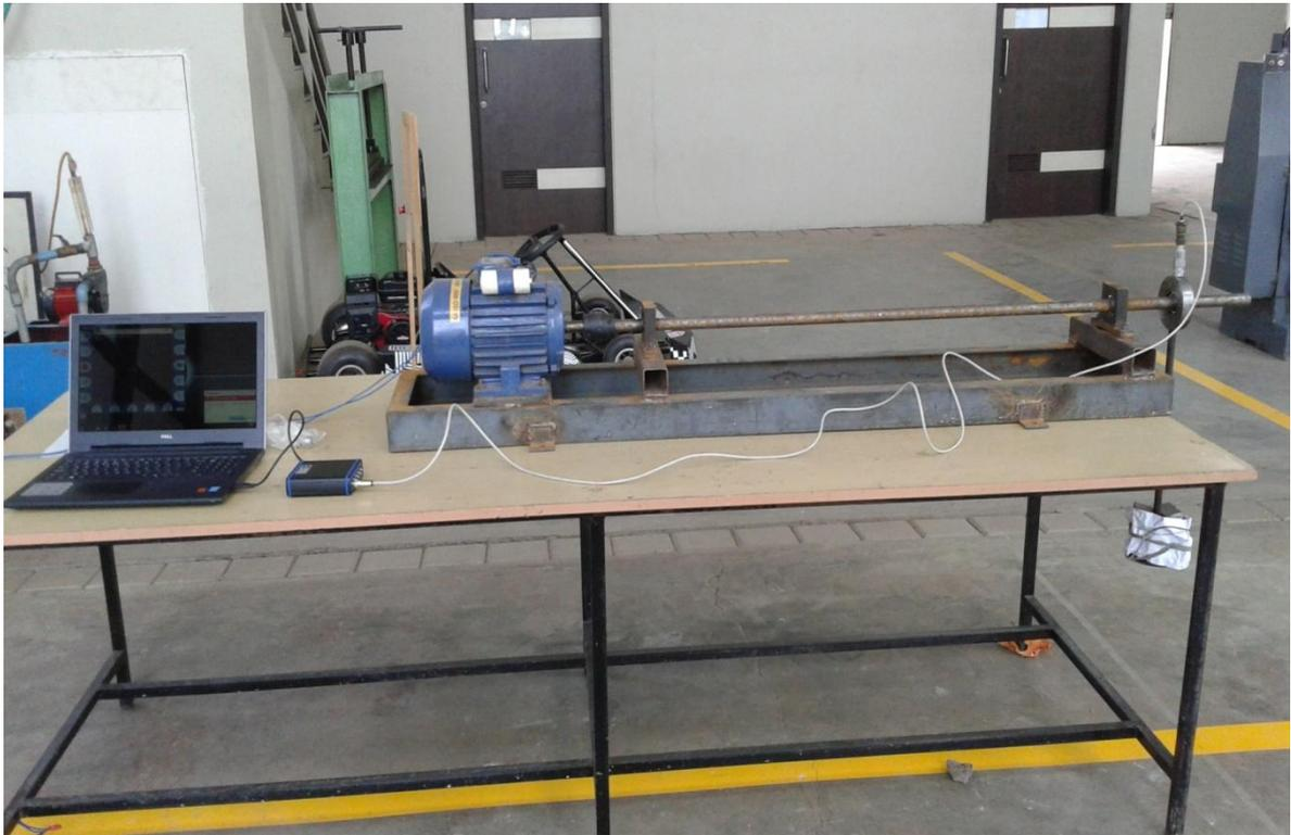
Fig. 1. Experimental Setup: Test rig of Defect detection analysis of Deep Groove Ball bearing
