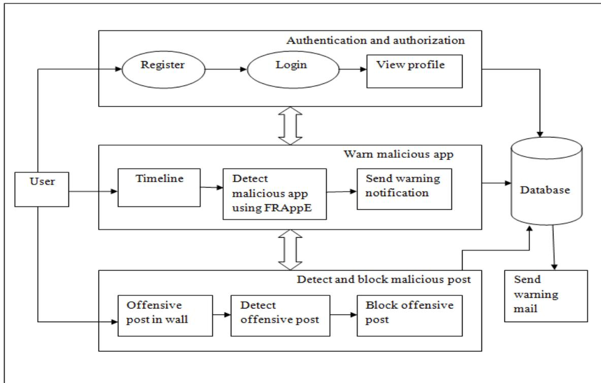
**Fig 2 System Architecture for proposed system**
