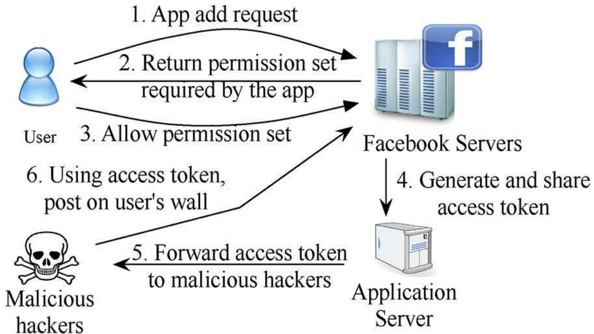
**Fig 1 System architecture for Existing system**
