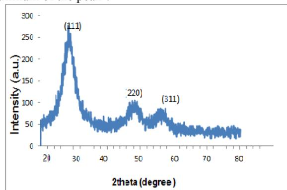
**Figure 1 . The X-ray diffractions of the colloidal ZnS nanoparticles**
