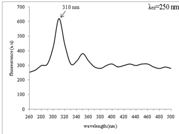
**Fig 4 : The Photoluminescence spectra of colloidal ZnS nanoparticles at room temperature.**
