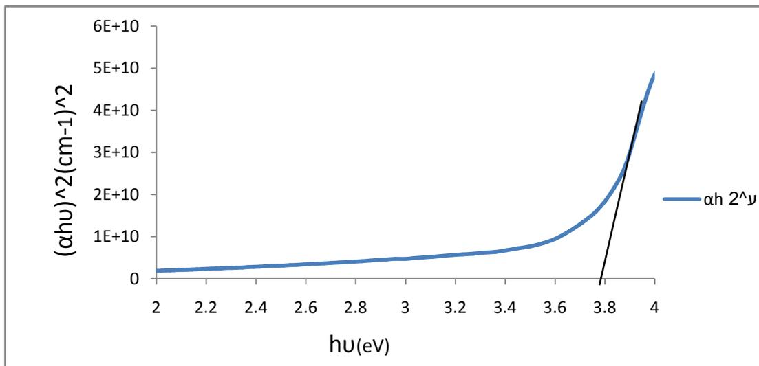
**Fig. 3. the graph between  $(\alpha h\nu)^2$  versus  $h\nu$  of ZnS nanoparticles .**
