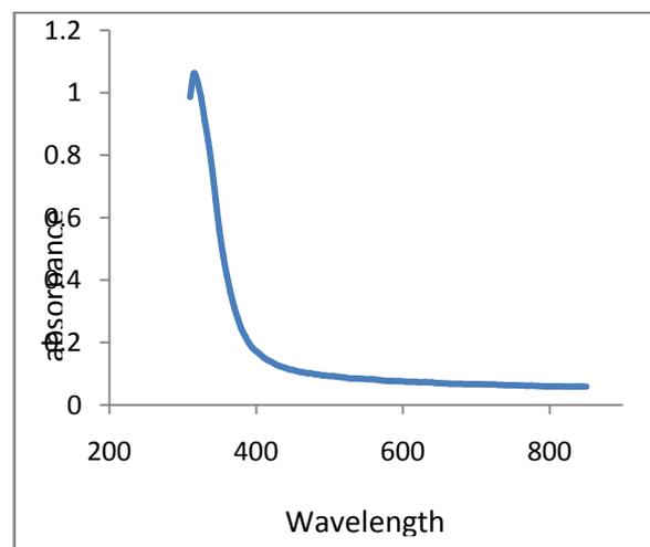
Fig:2 .UV-VIS absorption spectrum of ZnS nanoparticle.
