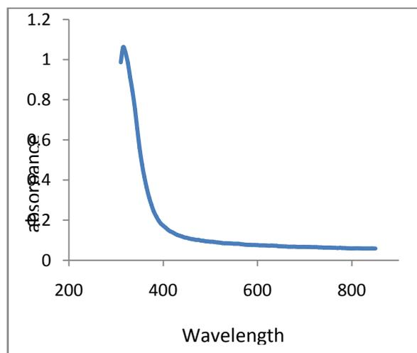
Fig:2 .UV-VIS absorption spectrum of ZnS nanoparticle.
