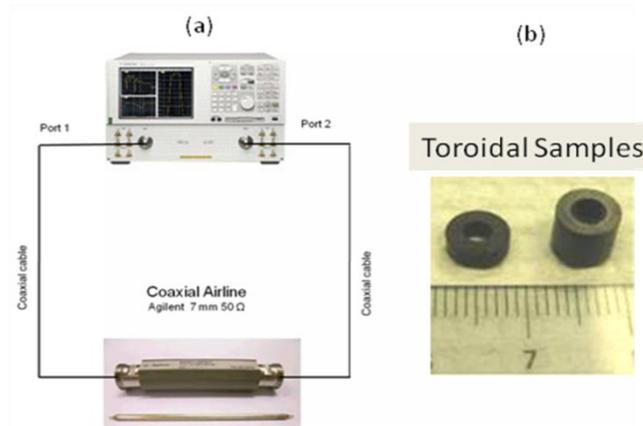
Figure 1: (a) Vector Network Analyser (VNA) for micro-wave measurements, (b) Samples
