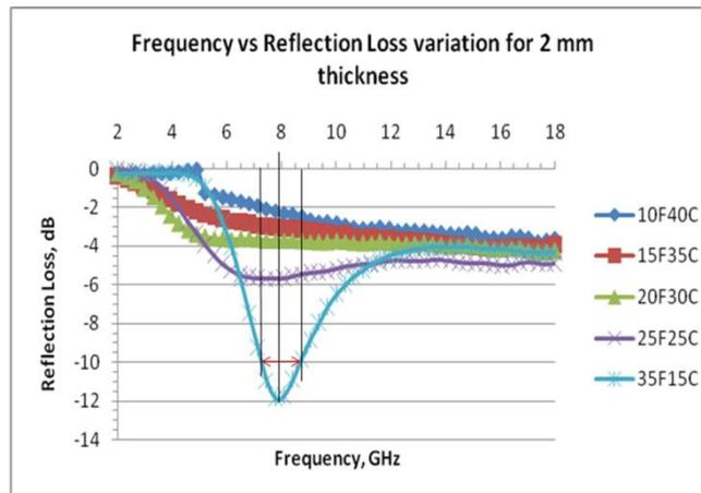
Fig. 5. Reflection loss ( $R_L$ , dB) vs. frequency (GHz) for  $t = 2.0$  mm for various compositions of Nano-Composites
