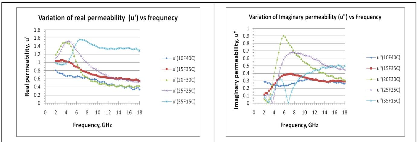
Fig. 4. Variation of (a) Real permeability ( $\mu'$ ) and (b) magnetic loss ( $\mu''$ ) with frequency (GHz) of nano-composite samples
