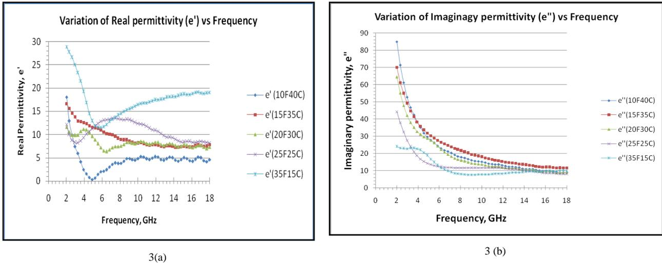
Fig. 3. Variation of the (a) Dielectric constant ( $\epsilon'$ ) with frequency (GHz) (b) Dielectric Loss ( $\epsilon''$ ) with frequency (GHz) of Nano MWCNT and nano NiZn ferrite /TPU matrix based nano-composites
