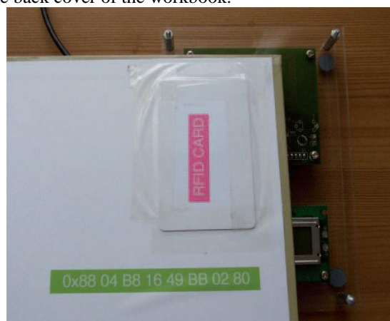
Figure 4. Workbook inside cover showing the RFID card (tag) used in the prototype
