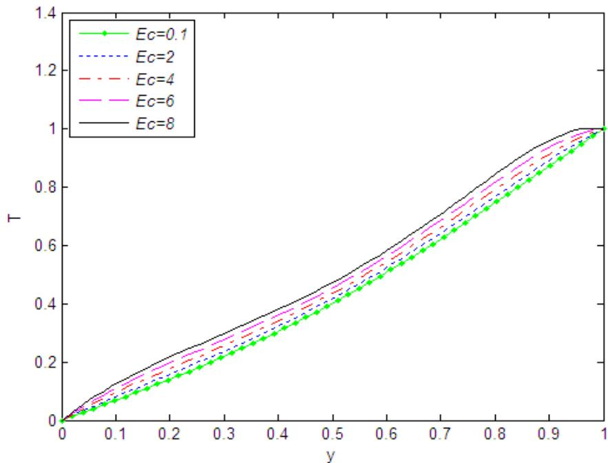
**Fig. 7:** Temperature distributions at various Eckert number  $Ec$  for fixed,  $Re = 1$ ,  $Gr = 3$ ,  $M = 2$ ,  $\phi = 45^0$  and  $Pr = 0.71$
