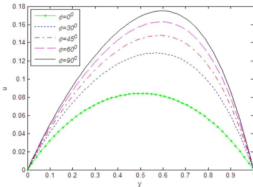
**Fig. 4:** Velocity distributions at various inclination angles  $\phi$  for fixed  $Re = 1$ ,  $Gr = 3$ ,  $M = 2$ ,  $Ec = 0.1$  and  $Pr = 0.71$
