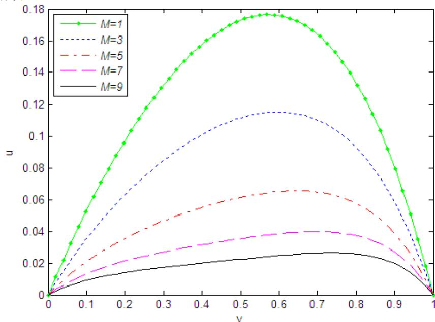
**Fig. 2:** Velocity distributions at various Hartmann number  $M$  for fixed  $Re = 1$ ,  $Gr = 3$ ,  $\phi = 45^\circ$ ,  $Ec = 0.1$  and  $Pr = 0.71$
