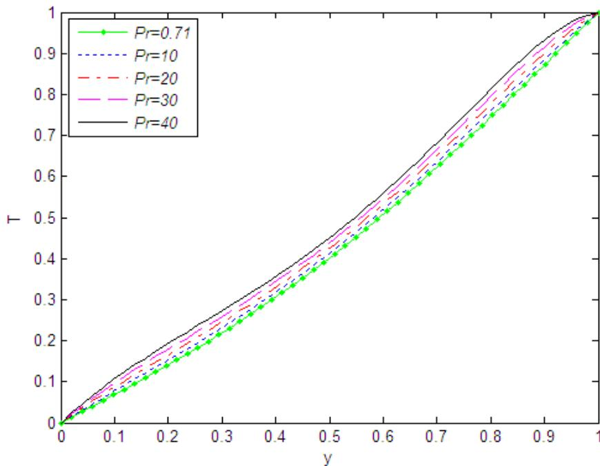
**Fig. 9:** Temperature distributions at various Prandtl number  $Pr$  for fixed  $Re = 1$ ,  $Gr = 3$ ,  $M = 2$ ,  $\phi = 45^0$  and  $Ec = 0.1$
