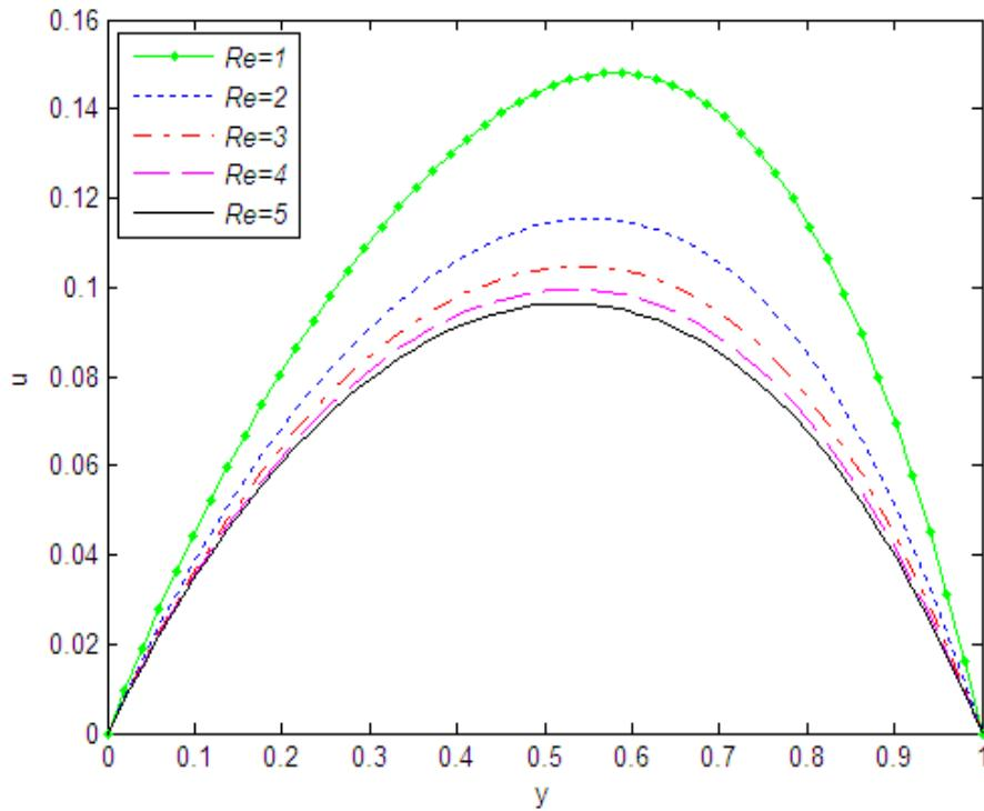
**Fig. 5:** Velocity distributions at various Reynolds number  $Re$  for fixed  $Gr = 3$ ,  $M = 2$ ,  $\phi = 45^0$ ,  $Ec = 0.1$  and  $Pr = 0.71$
