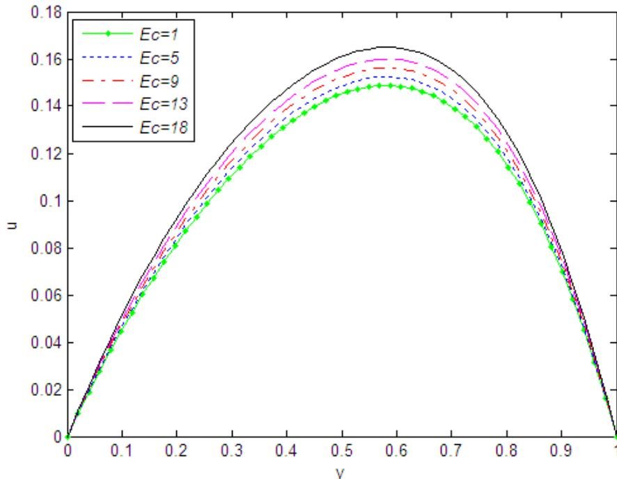
**Fig. 6:** Velocity distributions at various Eckert number  $Ec$  for fixed  $Re = 1$ ,  $Gr = 3$ ,  $M = 2$ ,  $\phi = 45^0$  and  $Pr = 0.71$
