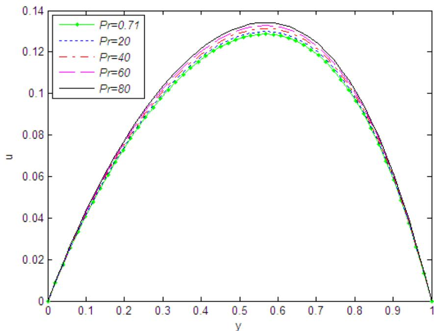
**Fig. 8:** Velocity distributions at various Prandtl number  $Pr$  for fixed,  $Re = 1$ ,  $Gr = 3$ ,  $M = 2$ ,  $\phi = 45^0$  and  $Ec = 0.1$
