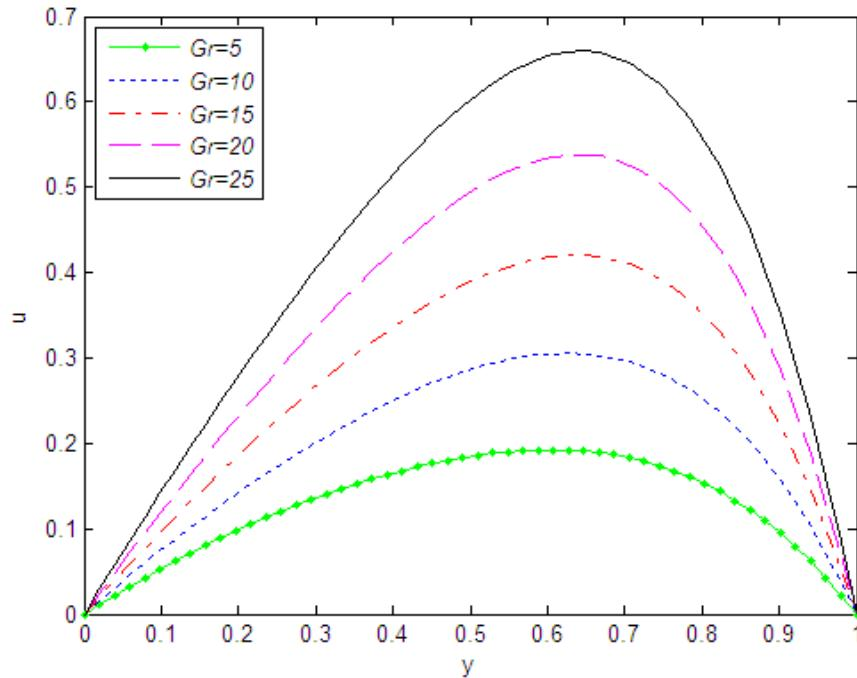
**Fig. 3:** Velocity distributions at various Grashof number  $Gr$  for fixed  $Re = 1$ ,  $M = 2$ ,  $\phi = 45^0$ ,  $Ec = 0.1$  and  $Pr = 0.71$
