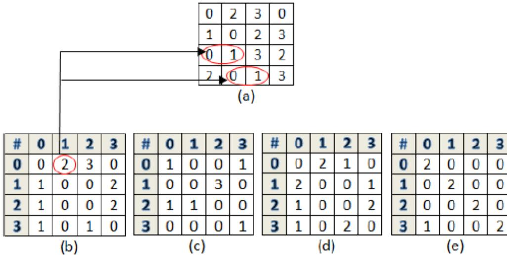
Fig. 2. GLCM construction based on a (a) test image along four possible directions (b) 0° (c) 45° (d) 90° and (e) 135° with a distance  $d = 0$ .
