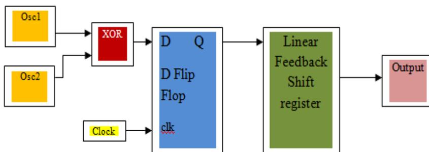
Fig. 3: Architecture of Proposed RNG
