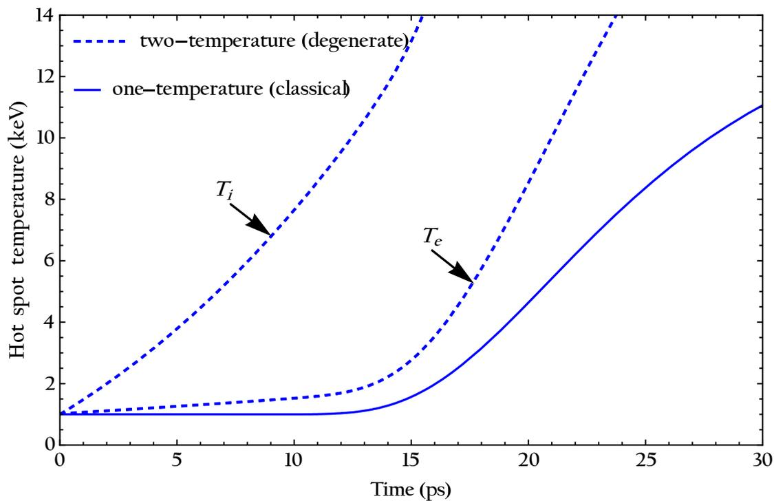
Fig.3. Time evolution of the hot spot temperature for two different plasma conditions: degenerate (dashed line) based on the nodal energy model and classical (solid line) based on the normal equation of power balance.
