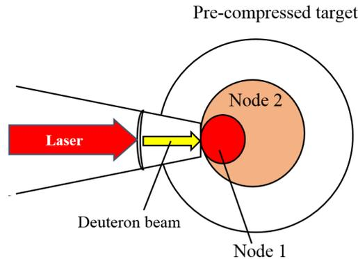
Fig.1. Fast ignition by the laser-accelerated deuteron trigger based on the two nodal technique.
