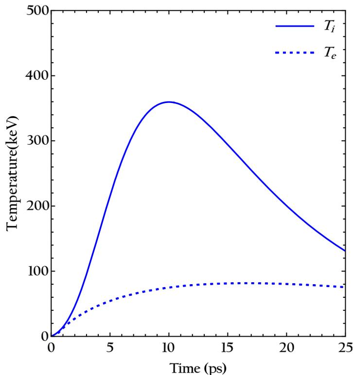
Fig.4. Temperature evolution of the ions (solid line) and electrons (dashed line) of a degenerate plasma vs. time. The calculations has been done based on the two nodal concept.
