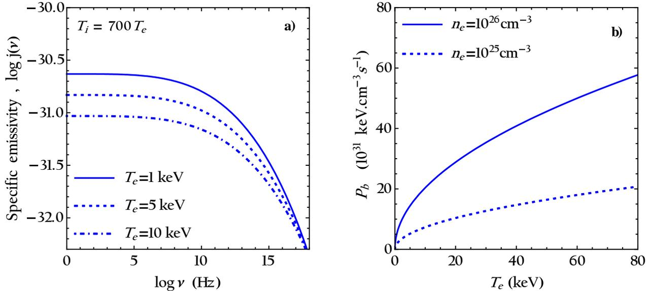
Fig.2. a) Specific emissivity of the Bremsstrahlung radiation in a degenerate DT plasma at,  $T_i = 700 T_e$ , as the ion temperature value and three different electron temperatures:  $T_e = 1$  keV (solid line),  $T_e = 5$  keV (dashed line) and  $T_e = 10$  keV (dashed-dotted line). b) The Bremsstrahlung radiation loss as a function of electron temperature and density,  $n_e$ .
