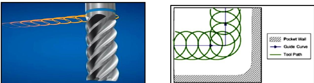
Figure 1. Trochoidal Milling
