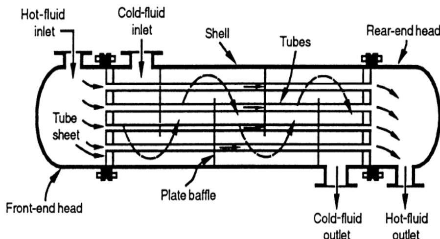
Fig.3.1 Shell-and-tube exchanger [10]
