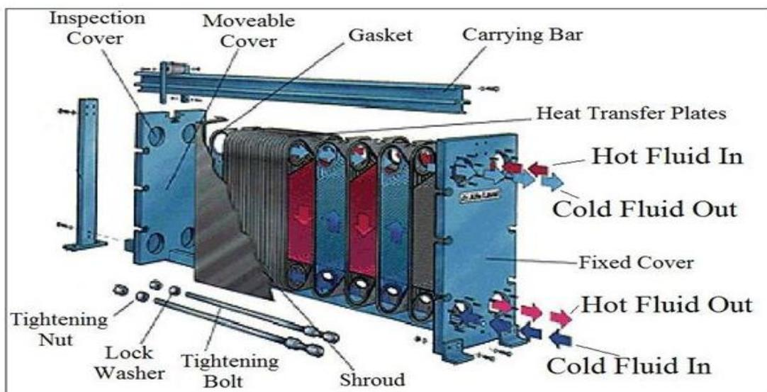
Fig.3.2 Plate heat exchangers [11]
