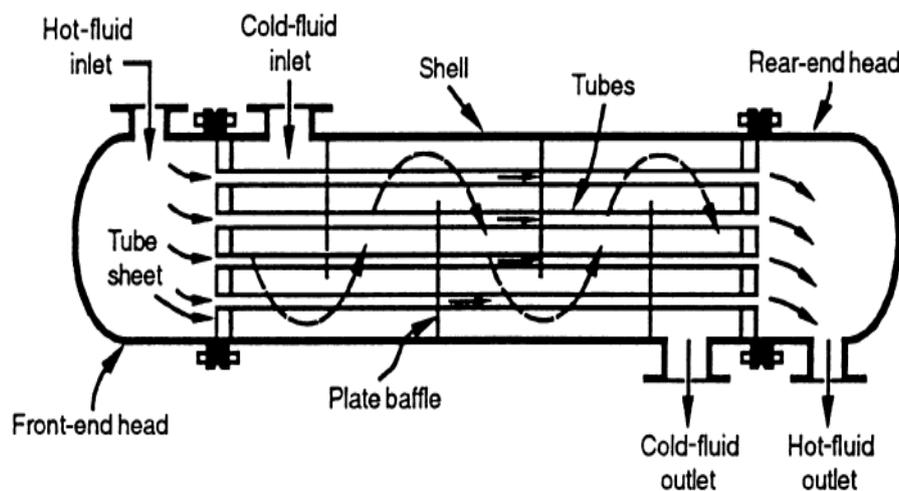
Fig.3.1 Shell-and-tube exchanger [10]
