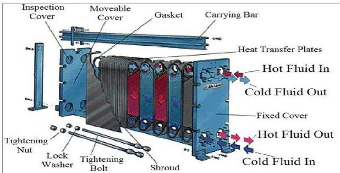
Fig.3.2 Plate heat exchangers [11]
