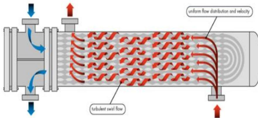
Fig.4.1 Twisted tube heat exchanger [9]
