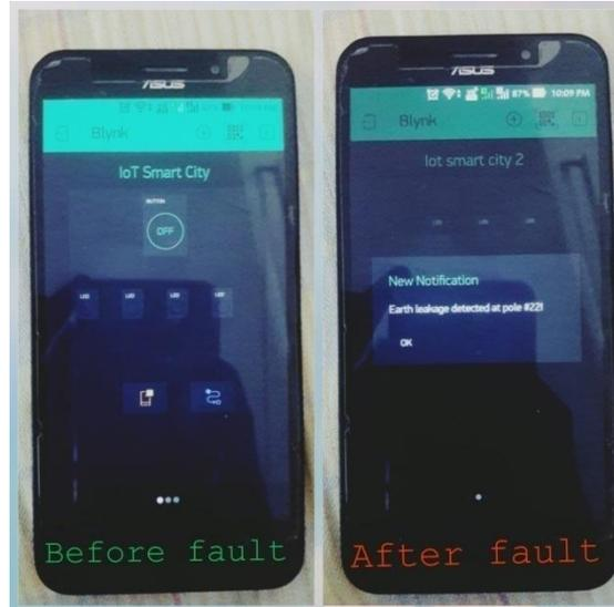
Fig. 3 Control and monitoring in an authenticated device.
