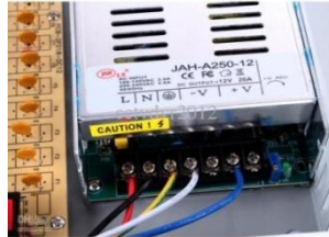
Fig 4. Power supply unit [8]
