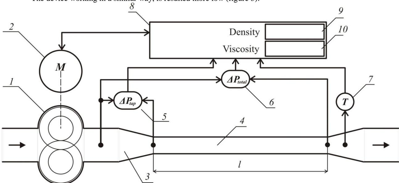
Figure3. Automatic capillary viscosimeter of the continuous act
