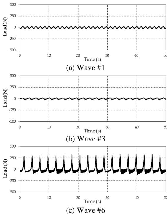
Fig. 3 Measured wave forces for multipile
