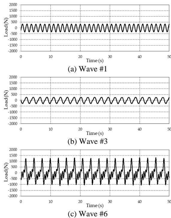
Fig. 4 Measured wave forces for hybrid
