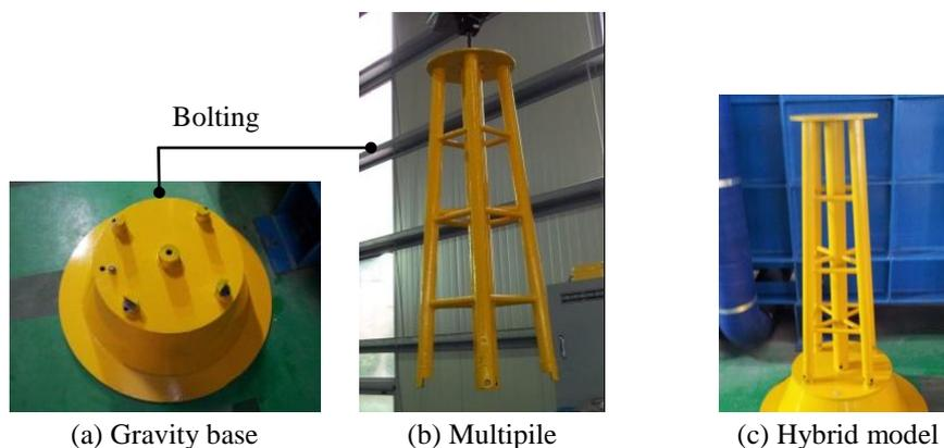
Fig. 1 Structural members assembling for test model
