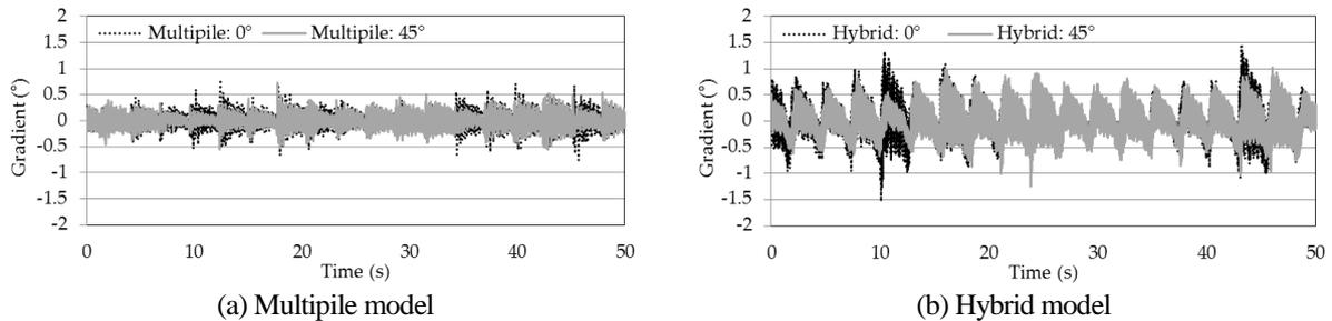
Fig. 8 Wave-induced vibration at extreme wave #6
