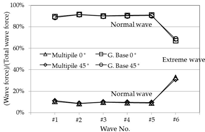
Fig. 9 Wave force percentages for the structural members
