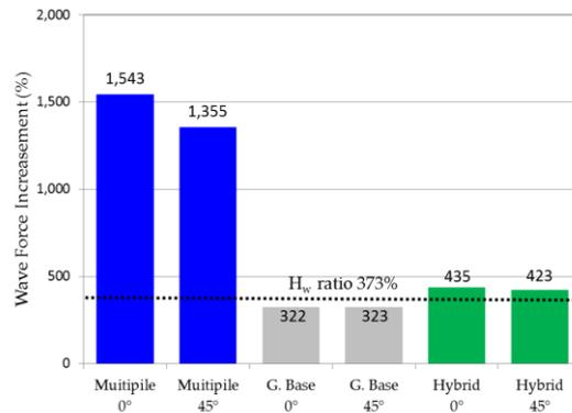
Fig. 6 Wave force at extreme wave
