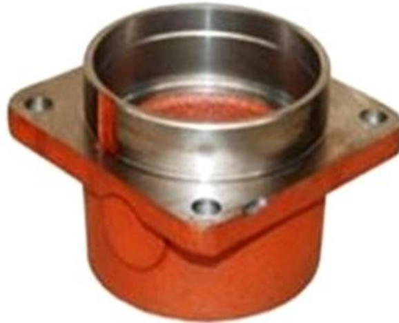
Figure 1.1. Bearing covers casting after machining
