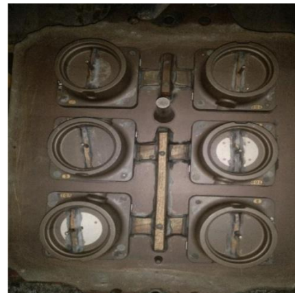
Figure 10. Bearing cover Modified pattern (Cope half)
