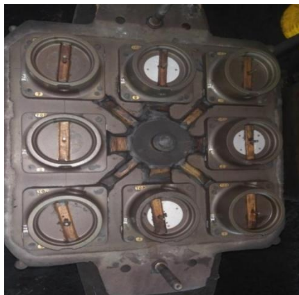
Figure 9. Bearing cover Old pattern (Cope half)
