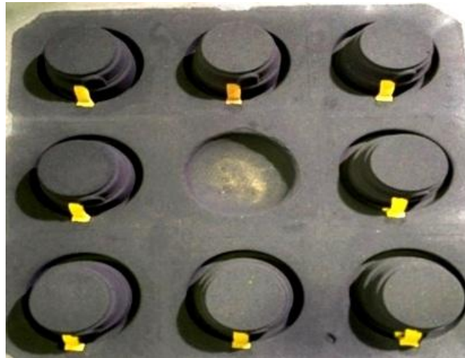
Figure 6. Drag half of Bearing cover mold box
