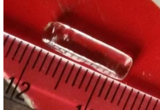
Figure.1 As grown single crystal of LSSC
