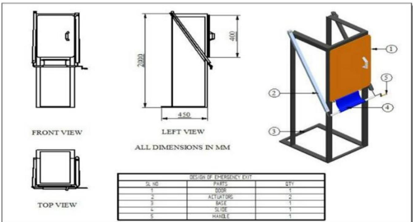
Fig 3. CAED Model of Pneumatically powered Emergency Exit System
