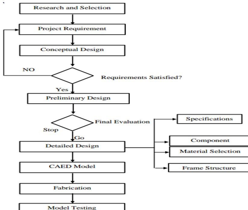
Fig.2 Design Process Flowchart
