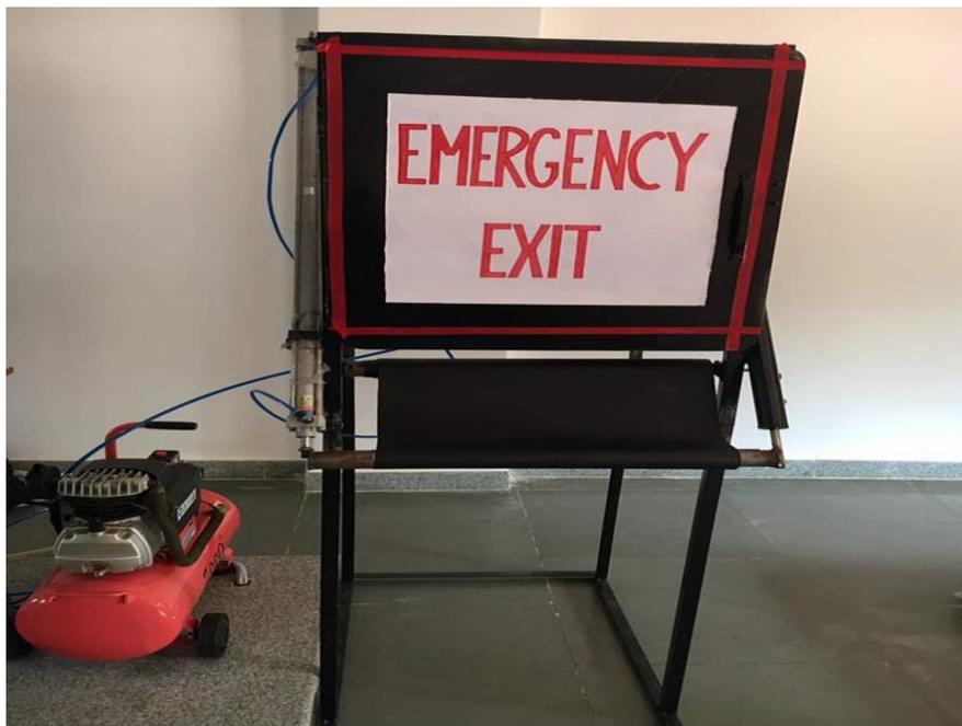
Fig.5 Fabricated model of Pneumatically operated Emergency Exit System
