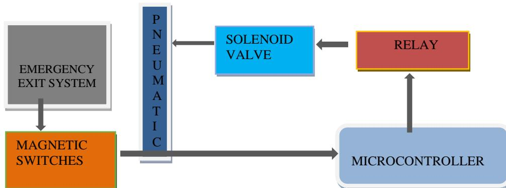
Fig 4. Block Diagram of Working Principle of Pneumatically Powered Emergency Exit System
