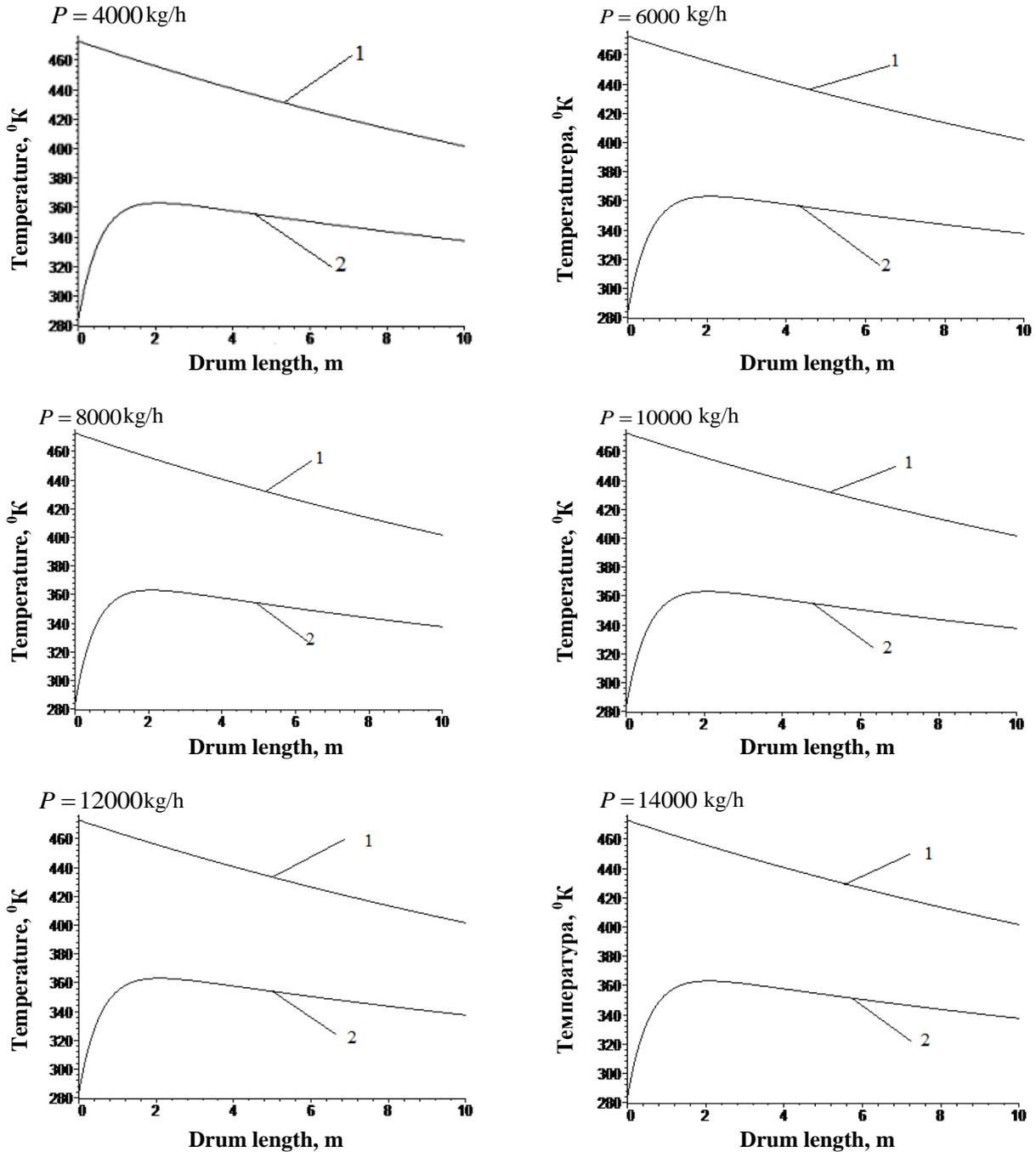
Fig.2. Changes in the temperature of the drying agent (1) and raw cotton (2) along the length of the drum
