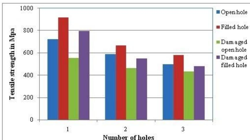
Fig 10 Analyses of tensile strength results of 1 hole, 2 holes and 3 holes in the specimens
