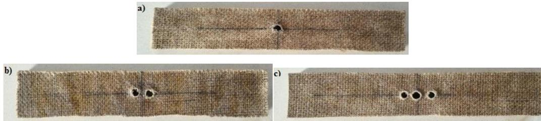
Fig 4 Number of holes in the damaged specimen along horizontal axis; (a) 1 hole, (b) 2 holes and (c) 3 holes
