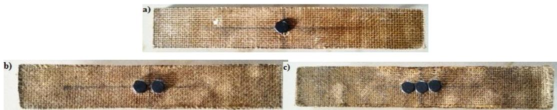
Fig 3 Number of holes in the specimen along horizontal axis is filled with M6 bolt and nut; (a) 1 bolt, (b) 2 bolts and (c) 3 bolts
