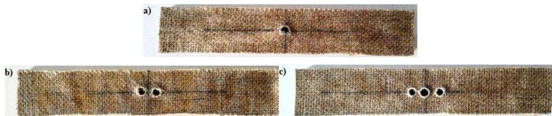
Fig 2 Number of holes in the specimen along horizontal axis; (a) 1 hole, (b) 2 holes and (c) 3 holes
