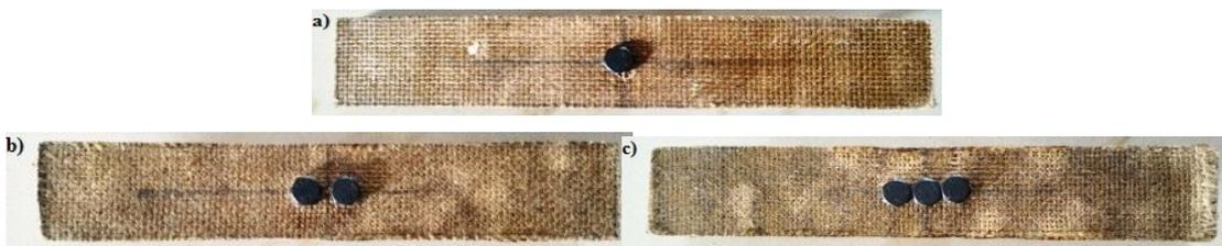
Fig 5 Number of holes in the damaged specimen along horizontal axis is filled with M6 bolt and nut; (a) 1 bolt, (b) 2 bolts and (c) 3 bolts
