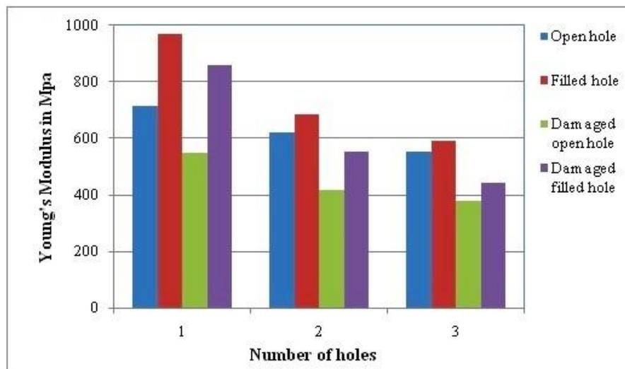
Fig 11 Analyses of modulus of elasticity results of 1 hole, 2 holes and 3 holes in the specimens.
