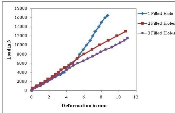
Fig 7 Load v/s deformation curve for specimens have 1 hole, 2 holes and 3 holes is placed with M6 bolt
