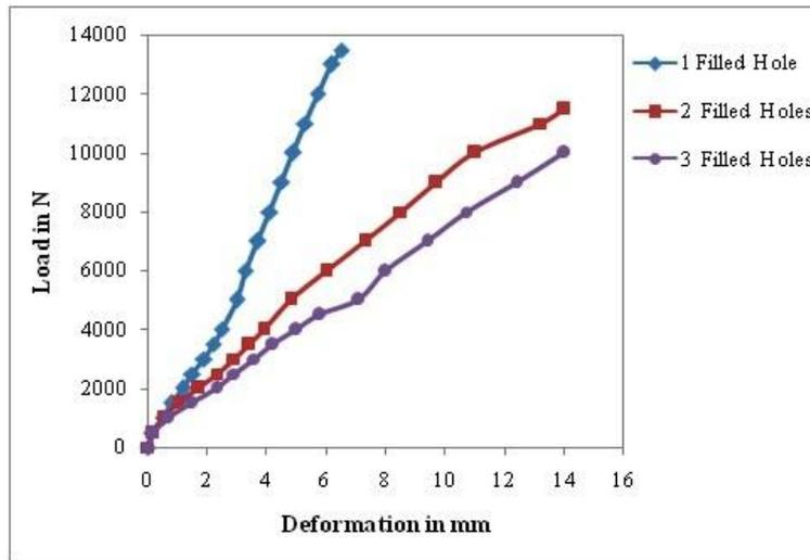
Fig 9 Load v/s deformation curve for damaged specimens have 1 hole, 2 holes and 3 holes is placed with M6 bolt
