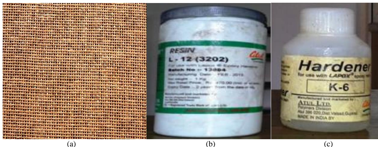
Fig.1 Raw materials used for composites: (a) jute fabric, (b) Lapox L-12 epoxy resin and (c) hardener k-6
