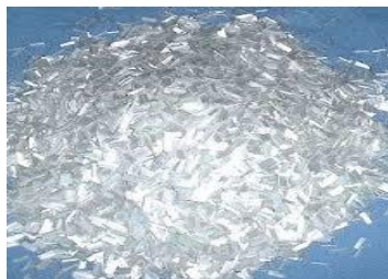
Figure 2: E-Glass Fibers (Chopped strands) Properties of E-Glass Fiber
