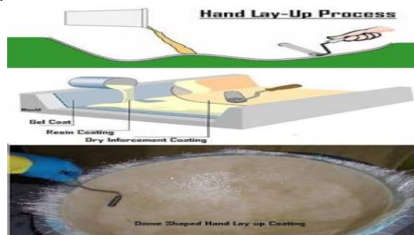
Figure 4: Hand Lay Up Technique
