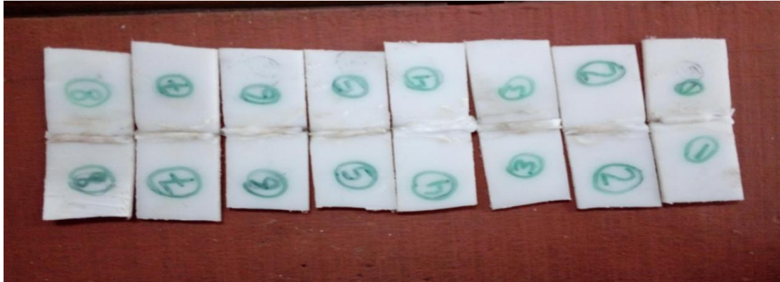
Figure 1 Weld bead formed in 1 to 8 th experiment
