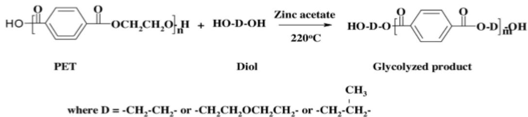
Fig 2: Glycolysis of PET waste <sup>(1)</sup>
