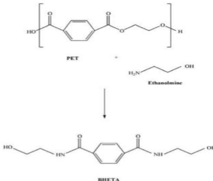
Fig 3: Aminolysis of PET waste <sup>(3)</sup>
