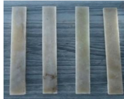
Fig2. Specimens of GFRP laminate with dimensions of 250 mm × 30 mm × 8 mm
