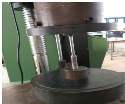
Fig 3: Compaction under CTM
