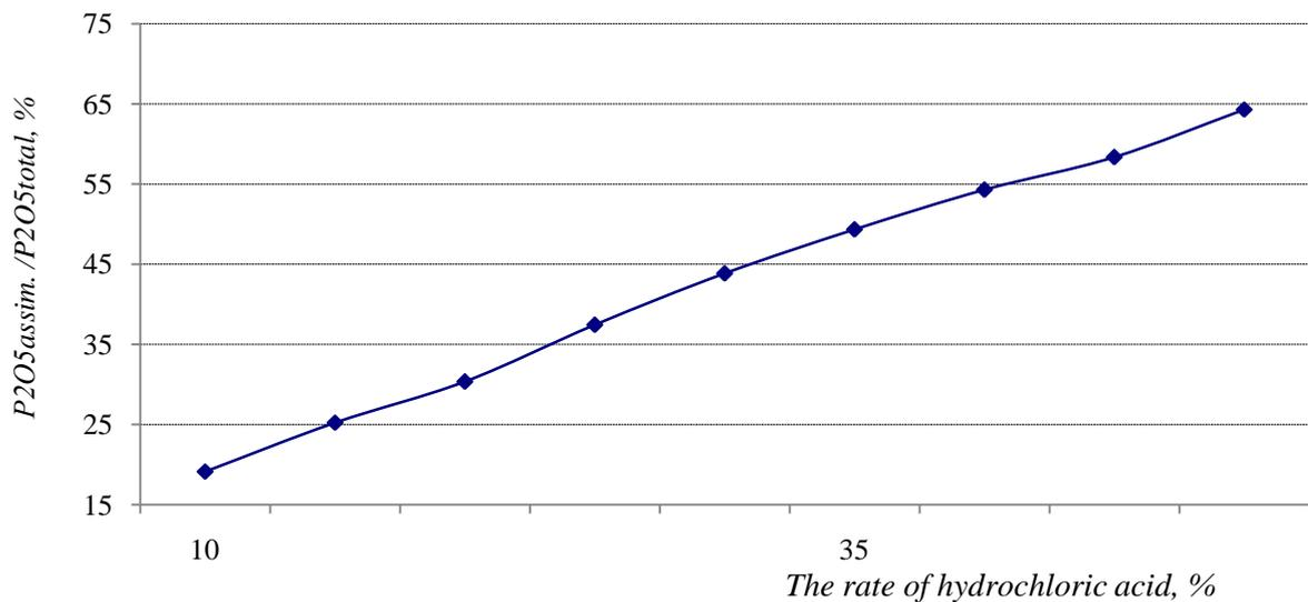
Fig. 3. Dependence of the relative content of assimilable forms of phosphorus on citric acid on the norm of hydrochloric acid.
