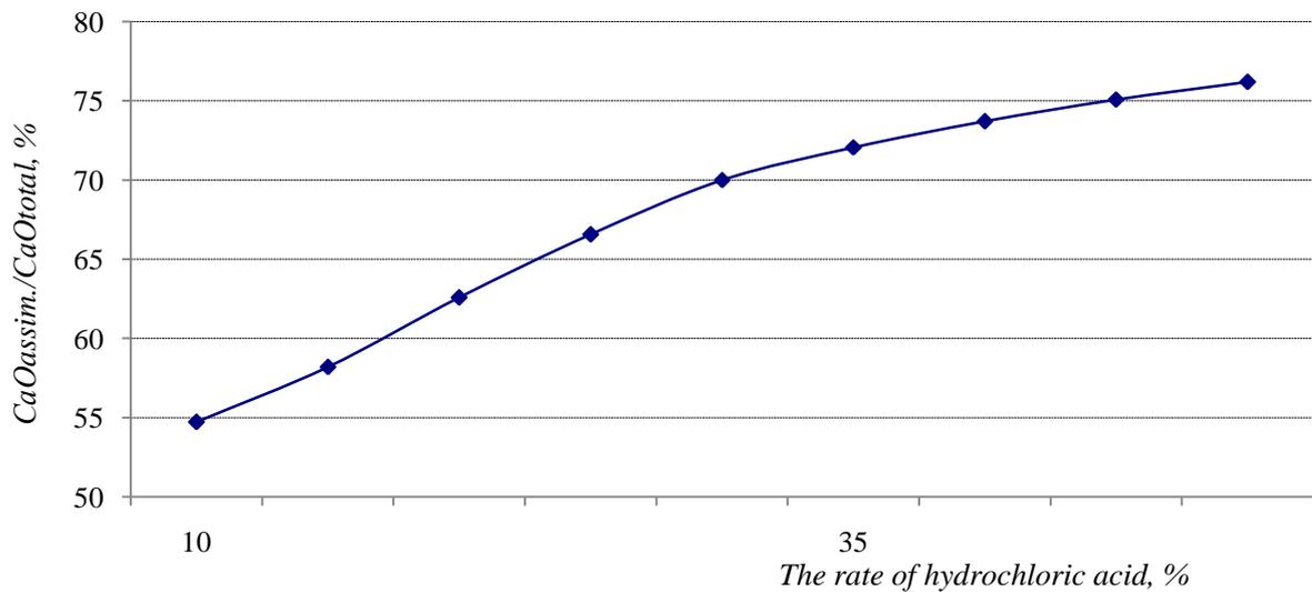
Fig. 4. Dependence of the relative content of assimilated forms of calcium on the norm of hydrochloric acid.
