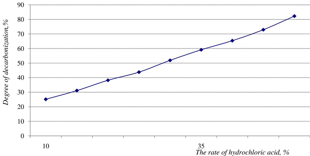
Fig. 1. Dependence of the degree of decarbonization of phosphate raw materials on the norm of hydrochloric acid.
