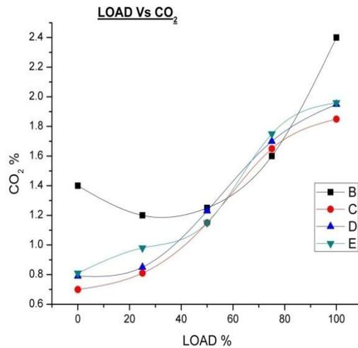
Figure 5.6 shows the variation carbon dioxide with respect to load for diesel fuel and Karanja biodiesel and additives. It is clearly seen that from graph all the blend shows low emissions of carbon dioxide at low loads and slightly increases at half loads which is negligible and again decreases at full loads when compared with conventional diesel
