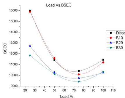
Figure 5.3 shows the variation of brake specific energy consumption with respect to load for diesel fuel and Karanja biodiesel and additives.It can be observed from the figure that shows B20 and B30 blends shows lower specific energy consumption when compared to the conventional diesel but B10 biodiesel blend shows higher specific energy consumption at low load. But after half load energy consumption decreases.
