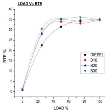
Figure 5.4 shows the variation of brake thermal efficiency with respect to load for diesel fuel and Karanja biodiesel and additives. It can be observed from the figure that all samples gave good performance than diesel around 12% average increase in BTE occurred in all samples when compared to diesel. This is because of excess oxygen content in the Karanja oil and because of combustion enhancer additive(EHN). B30 gave reasonable performance among all the
