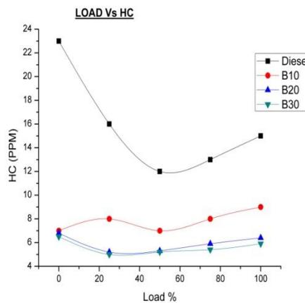
Figure 5.7 shows the variation hydrocarbons with respect to load for diesel fuel and Karanja biodiesel and additives. Due to the excess oxygen present in the biodiesel complete combustion took place and formation of HC gone down. From the graph it is clear that B30 showed least HC production.
