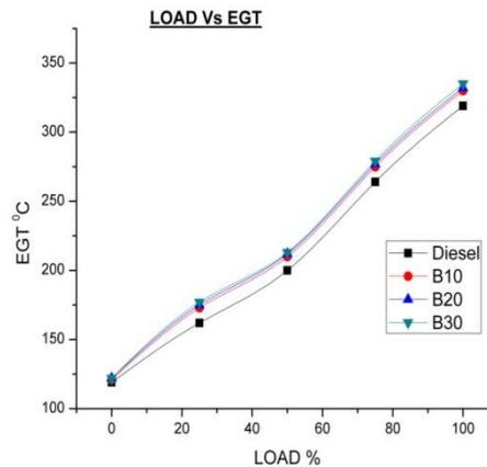
Figure 5.8 shows the variation exhaust gas temperature with respect to load for diesel fuel and Karanja biodiesel and additives. It is a measure of performance as higher exhaust gas temperatures results in higher heat release in combustion chamber there by giving probability to increase brake thermal efficiency. From the graph it is clearly seen that that EGT is high in all the blends when compared to conventional diesel.
