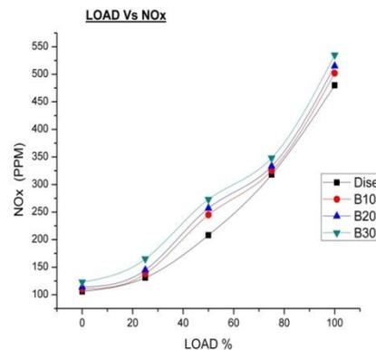
Figure 5.9 shows the variation of NOx with respect to load for diesel fuel and Karanja biodiesel and additives. Due to the excess oxygen present in the biodiesel complete combustion took place and temperature inside the combustion chamber increased thereby increasing the NOx emission. From the graph it is clear that B30 showed maximum NOx emissions. It cannot be completely stopped but it can be minimized like EGR techniques.
