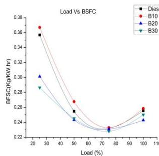
Figure 5.2 shows the variation of brake specific fuel consumption with respect to load for diesel fuel and Karanja biodiesel and additives.It can be observed from the figure that shows b20 and b30 blends shows lower specific fuel consumption when compared to the conventional diesel But b10 biodiesel blend shows higher specific fuel consumption at any load. so should prefer b10 when for lower fuel consumption
