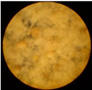
Fig. 5. Large pieces of calcite are noted in the control variant (an increase of 150 times).
