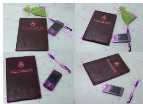
Fig. 2 Comparison of feature points extraction between Harris and SIFT
