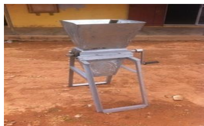
Fig9: The constructed manually operated cassava grater
