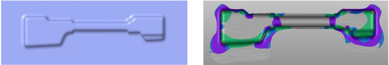
Figure: 5 Iteration A Stage 1 Die surface and Formability Analysis
