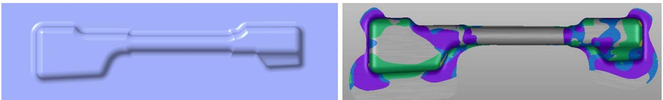
Figure: 6 Iteration A Stage 2 Die surface and Formability Analysis
