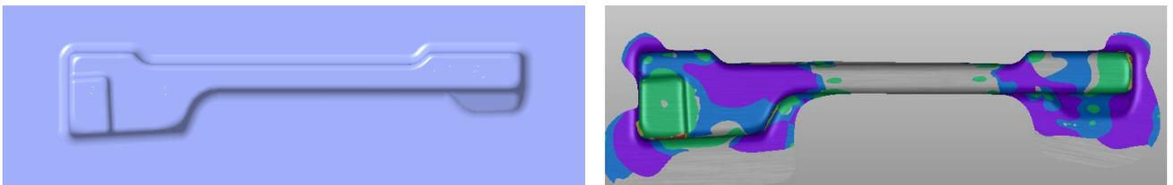
Figure: 7 Iteration A Stage 3 Die surface and Formability Analysis
