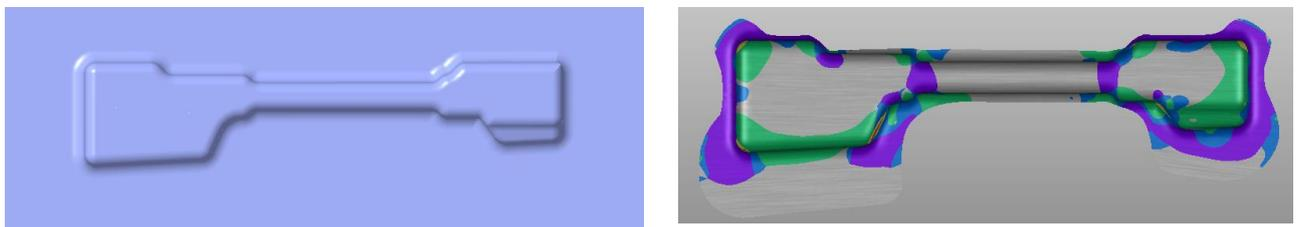
Figure: 10 Iteration B Stage 2 Die surface and Formability Analysis
