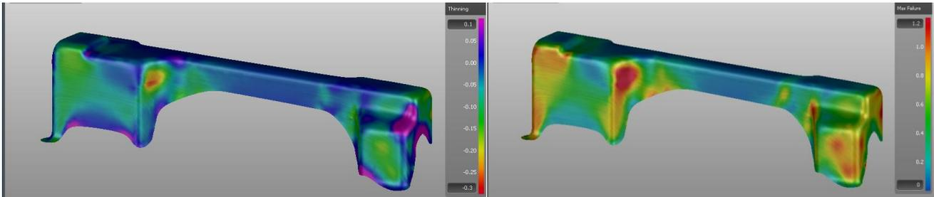
Figure: 14 Iteration B Stage 5 Thinning and Maximum Failure Analysis
