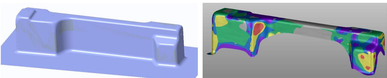
Figure: 13 Iteration B Stage 5 Die surface and Formability Analysis
