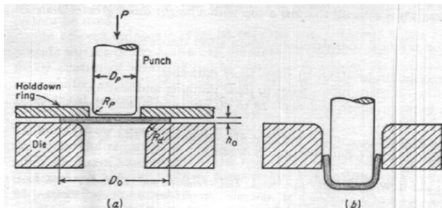
Figure: 1 Deep Drawing of a cylindrical cup (a) before drawing (b) after drawing [2]
