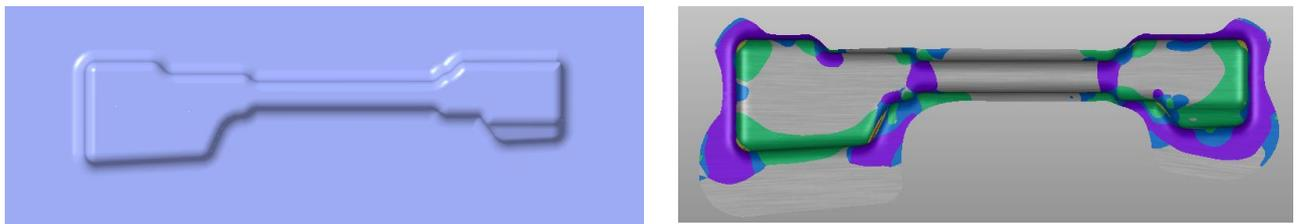
Figure: 11 Iteration B Stage 3 Die surface and Formability Analysis
