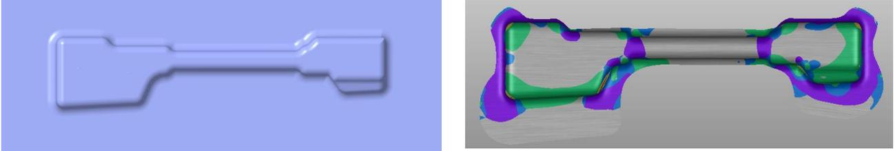
Figure: 9 Iteration B Stage 1 Die surface and Formability Analysis
