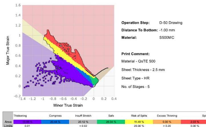
Figure: 15 Forming Limit Diagram (FLD) for Iteration B Stage 5
