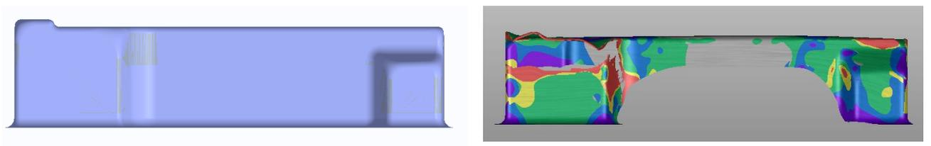
Figure: 8 Iteration A Stage 4 Die surface and Formability Analysis
