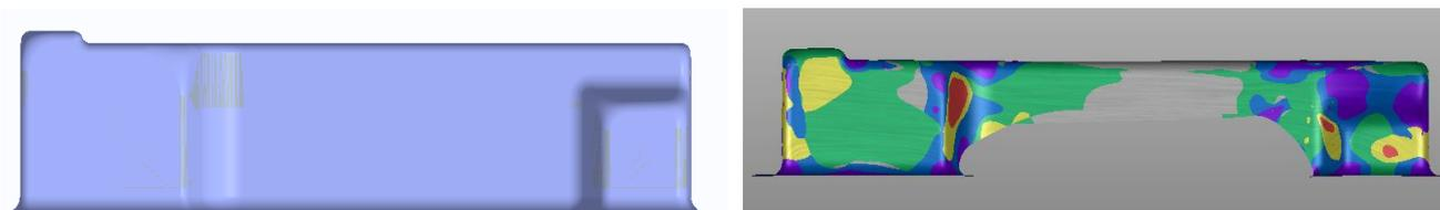
Figure: 12 Iteration B Stage 4 Die surface and Formability Analysis
