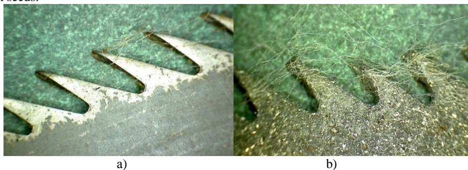
Fig.6. The exciting ability of the teeth of the saw blade: untreated (a) and treated with a stream of abrasive (b)
