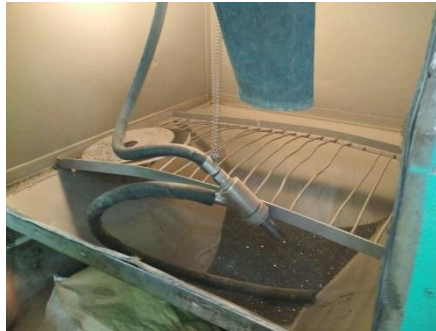
Fig. 4. Abrasive blasting chamber with ejector method of transporting the abrasive to the nozzle
