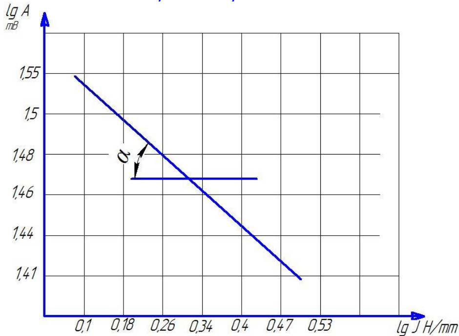
Figure 5. Log-log graph of the relationship of the vibro-acoustic signal to the stiffness of the workpiece. Material steel 40x, V = 120 m / min, S = 0.2 mm / rev, t = 1mm
