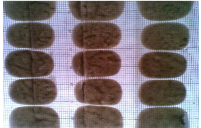
Fig. 6. The pattern of spots of deposited dust from corona needles 20 mm long, with their corridor arrangement and the distance between the needles in rows is twice as large as the distance between the needles in rows
