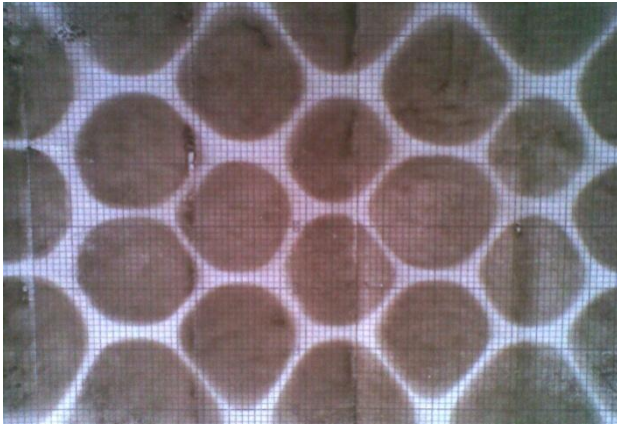
Fig. 5. The pattern of spots of deposited dust from corona needles 25 mm long, with their staggered arrangement and the same distance between the needles in the rows and between the rows of needles.
