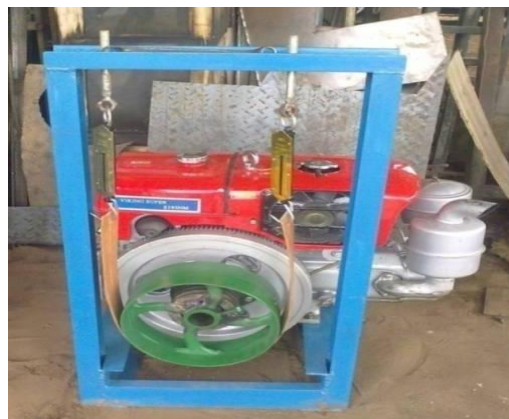
Plate 1. Locally Fabricated Prony Brake Dynamometer.
