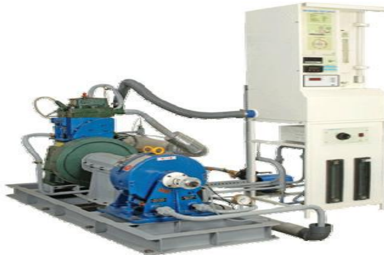
fig. 2 single cylinder 4-stroke diesel engine
