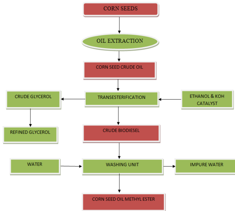
Fig.1 Biodiesel production flow chart
