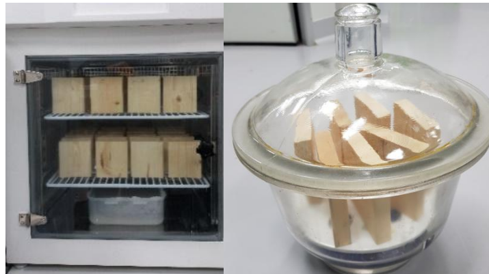
Fig 2. Moisture conditioning and drying process based on aqueous solution and oven drying method
