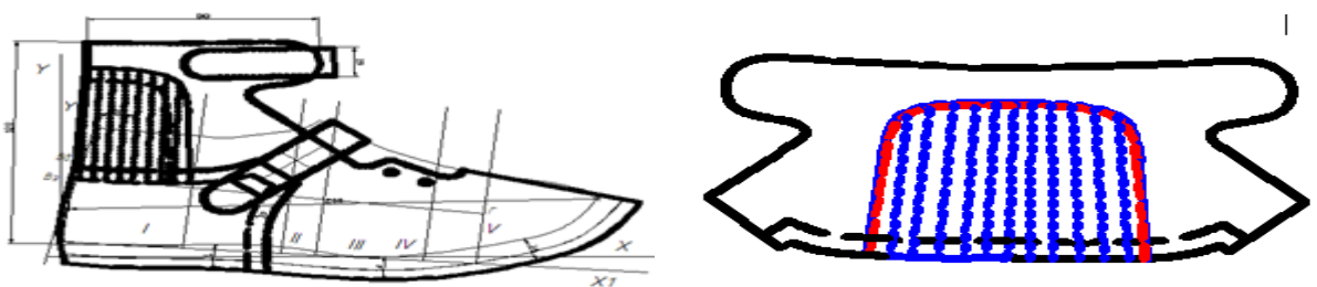
Figure 2 - The pattern design of the upper part of children's shoes
