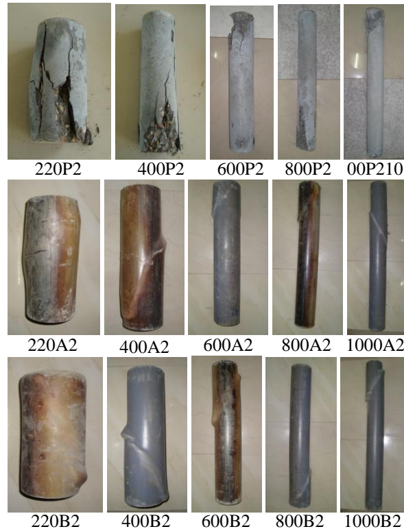
Fig. 7: Failure modes of specimens
